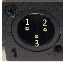
Figure 5: Audio Output Connector Pinout
