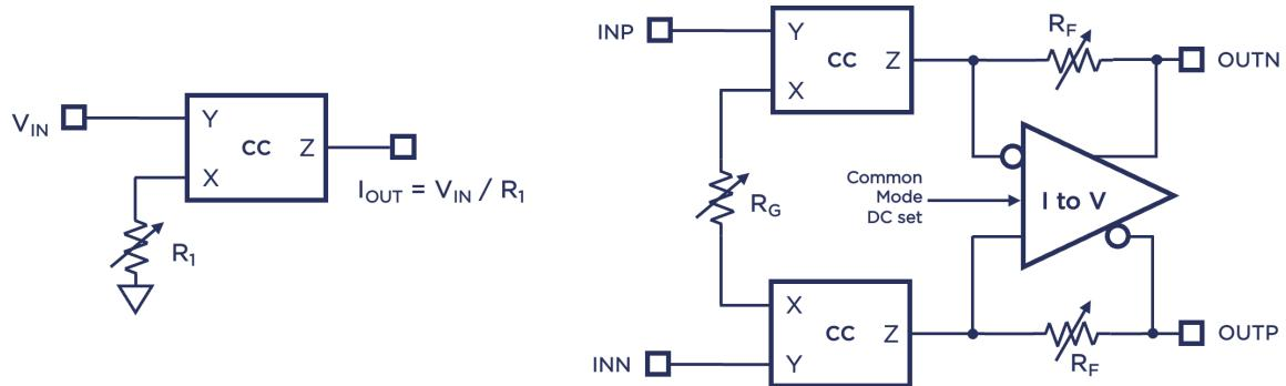
The Current Conveyor block is shown on the left, with the signal transfer function. The block diagram on the right shows how the CC blocks are used in conjunction with a differential current-to-voltage 2nd stage within the TS5510 IC.
