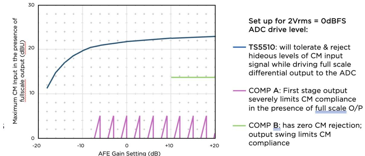
The graph shows the amount of VCM signal (ref. to GND) that these ICs can accommodate while supporting a 2Vrms differential output. The TS5510 exhibits more than 10X more CM compliance than the nearest competitor. This extends the “small signal” CMRR capability to apply to “large signal” events & interference that previously only transformer-coupled designs could tolerate.
