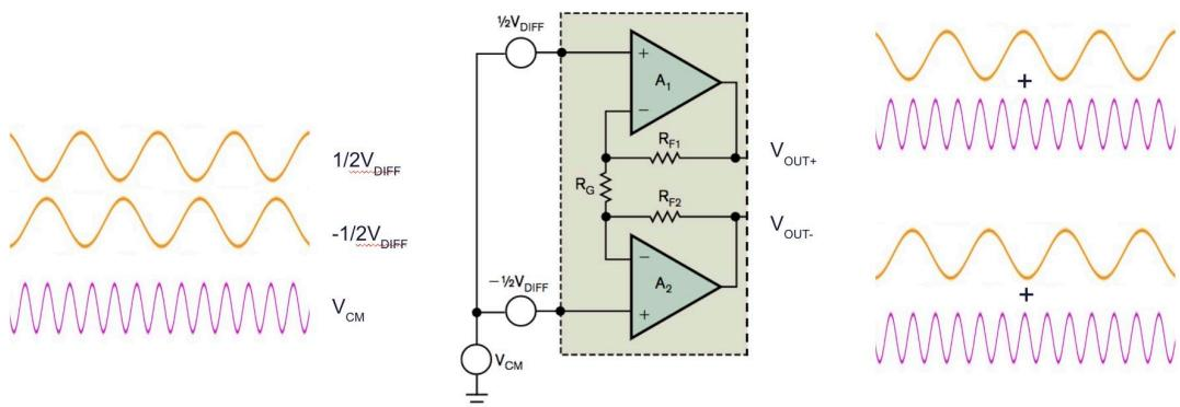
Traditional INA first stage, consisting of two amplifier blocks ( $A_1$  and  $A_2$ ) and gain setting resistors. Any CM on the input is passed through to subsequent circuitry.
