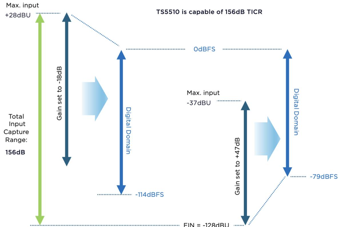
Example: +10dBu out of TS5510 = 0dBFS input for ADC
